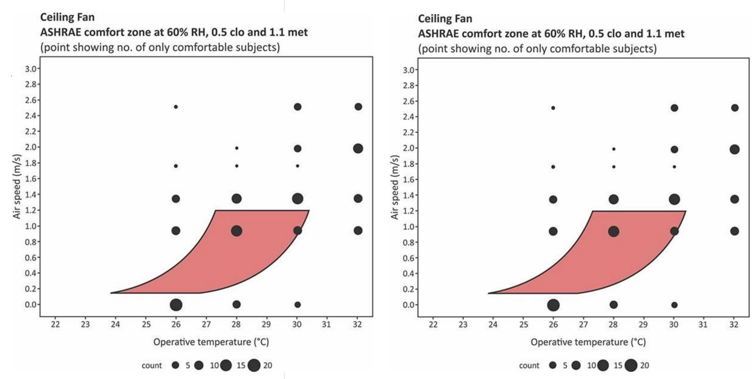
Ceiling fan Comfortable temperature, RH and selected air speeds against the ASHRAE comfort zone at 60% and 80% RH with elevated air movement
