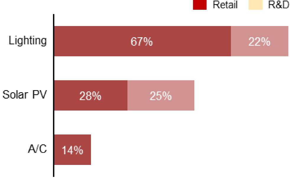
Compared to other energy technologies, the AC industry has made little progress in approaching maximum theoretical efficiency
