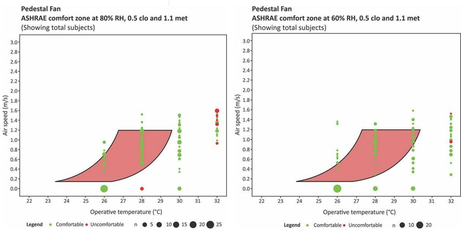
Pedestal fan Comfortable temperature, RH and selected air speeds against the ASHRAE comfort zone at 60% and 80% RH with elevated air movement
