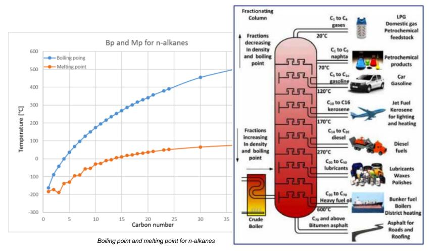
Typical hydrocarbon fractions from an oil refinery
