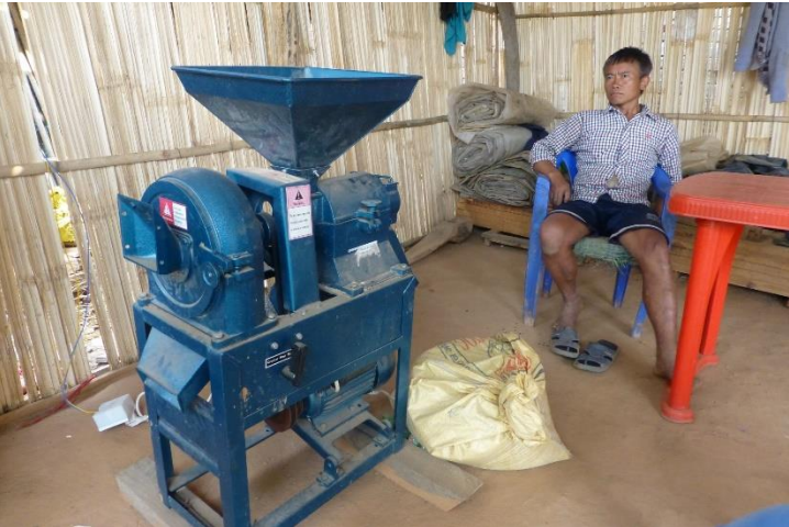
Grinding Mill – 1.8 kW
