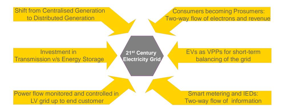
Two-way flow of electrons, information and revenue is making the grid more complex! Increased automation and IT is leading to a more vulnerable grid prone to cyber attacks.
