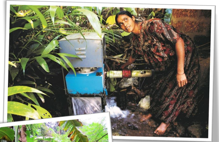
Pico Hydro Electricity Generating Systems in western Karnataka state in southwest India (one of many).
