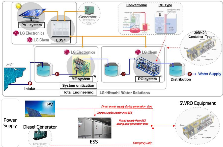
1) PV : Photovoltaic, 2) ESS : energy Storage System 3) MF : pretreatment(Microfiltration/Ultrafiltration) by Dual Media Filter 4) RO : Reverse Osmosis
