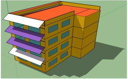
After high insulation window: Heating load: 33,694 kWh-> 12,406 kWh (63%) decrease, with outer shading: cooling load 43,083kWh ->38,028 kWh(shading coef. :0.7), 35,556 kWh (shading coef.: 1) decrease Therefore, Totally 76,777 kWh-> 47,962 kWh(shading coef: 1), 50,434 kWh(shading coef.:0.7), respectively 38% and 34% energy conservation
