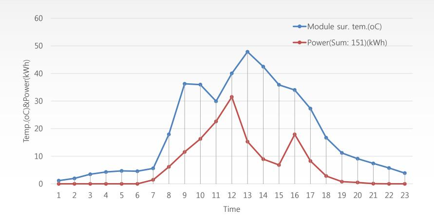
Photovoltaic system as a shading device in conjunction with Heating & cooling system PV power: 134 kWh -> 151 kWh (11.3% increase) Payback period: 5 year
