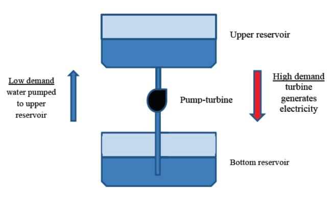
Figure 2 - Pumped storage hydroelectric station - basic principle of operation (Andrews, 2013, p. 342)
